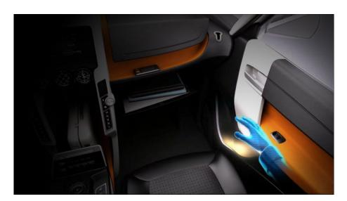
The centre console has also been developed to improve comfort and usability for the driver. Visteon have integrated a power sliding console which the driver can position to suit, and which is ergonomically designed for the user to rest their hand while controlling the functions on the console.
